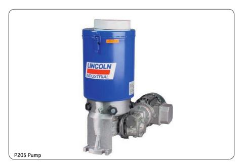
The P205 centralized lubrication pump is a high pressure multi-line pump that can drive up to 5 elements and is used in progressive automated lubrication systems. It is capable of handling direct supply of lubrication points or can be used as a centralized lubrication pump in larger progressive systems.
